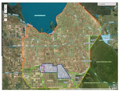
Controlling the water flow in and out of Lake Okeechobee is a complex process. To help limit the amount of water that is sent to the east and west estuaries, the state designated two areas of land within the Everglades Agricultural Area (highlighted in blue) to help with water storage and cleanup prior to it being sent to Everglades National Park.
