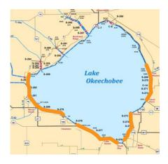
The Herbert Hoover Dike, outlined in orange, is one of the most important flood control structures in the state, enclosing much of Lake Okeechobee's 720 square miles and rising to an average height of 30 feet. It is currently undergoing an extensive rehabilitation process due to its age, however, this process is on schedule to end in 2022.
